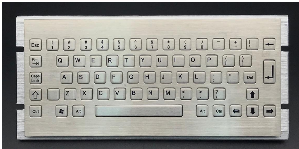
Product Code MKA-64 Mate Keyboard, Metal, 64 keys, Panel Mounted
